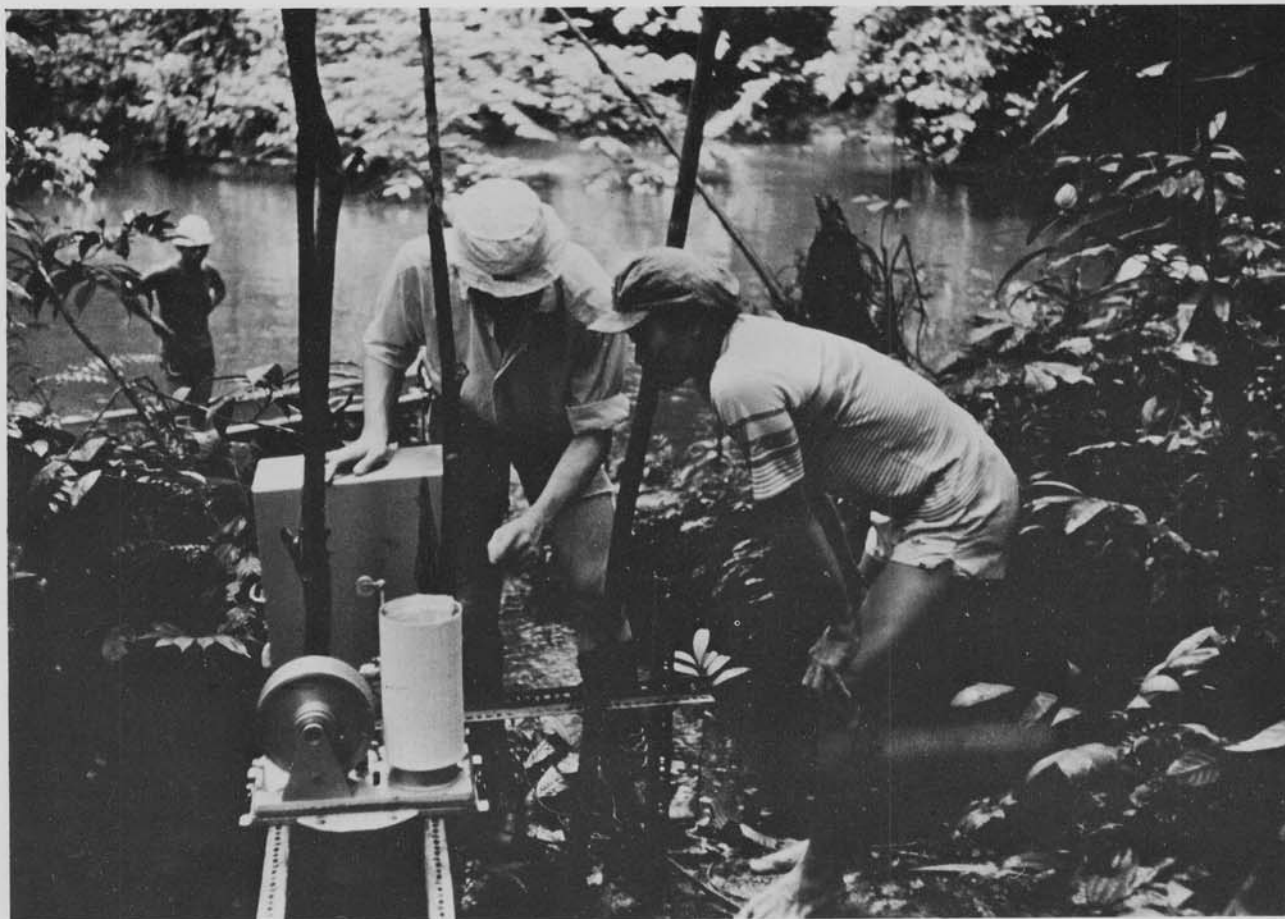
Hans Friederich explains the operation of a constant recording water level meter to Park Warden Siduck (P. Smart)
